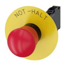
EMERGENCY STOP mushroom-type actuator, 22 mm, round, plastic, red, 40 mm, positive latching, according to EN ISO 13850, rotate-to-unlatch, with yellow backing plate, inscription: NOT-HALT, with holder, 1 NO+1 NC, screw terminal
