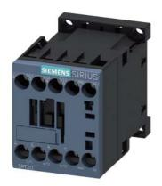
power contactor, AC-3e/AC-3, 7 A, 3 kW / 400 V, 3-pole, 48 V AC, 50/60 Hz, auxiliary contacts: 1 NO, screw terminal
