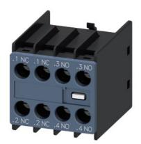
Auxiliary switch on the front, 2 NO + 2 NC Current path 1 NC, 1 NC, 1 NO, 1 NO for 3RH and 3RT screw terminal .1/.2, .1/.2, .3/.4, .3/.4
