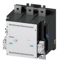
Contactor, Size 14, 3-pole, AC-3, 450 kW, 400/380 V (690 V) Auxiliary switch 44 (4NO+4NC) AC operation 200...240 V AC 50/60 Hz
