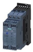
SIRIUS soft starter S2 63 A, 37 kW/500 V, 40  $^{\circ}\text{C}$  400-600 V AC, 24 V AC/DC Screw terminals Thermistor motor protection
