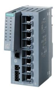
SCALANCE XC208G managed Layer 2 IE switch; IEC 62443-4-2 certified; 8x 10/100/1000 Mbps; RJ45 ports; 1x console port; diagnostics LED; redundant power supply; temp. range -40 °C to +70 °C; mounting: DIN rail/S7 mounting rail/wall redundancy functions; Office features (RSTP, VLAN,...); PROFINET IO device; Ethernet/IP-compliant; C-plug slot;
