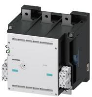
Contactor, Size 14, 3-pole, AC-3, 335kW, 400/380 V (690 V) Auxiliary switch 44 (4NO+4NC) AC operation 200...240 V AC 50/60 Hz
