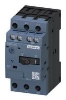
Circuit breaker size S00 for motor protection, CLASS 10 A-release 1.4...2 A N-release 26 A Screw terminal Standard switching capacity with transverse auxiliary switch 1 NO+1 NC
