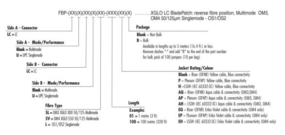
Note: Polarity CFP (Continuous fibre position) is available as an option. Remove the first dash "-" and add C to the end of the part number. Example: FBPLCLC5L-(XX)AQC
