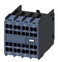
auxiliary switch front-side, 2 NO + 2 NC current path 1 NO, 1 NC, 1 NC, 1 NO for contactor relays size S00 spring-loaded terminal 53/54, 61/62, 71/72, 83/84 physically coded; only combinable with contactor relays 3RH2140\* and 3RH2440\* (according to EN 50011)
