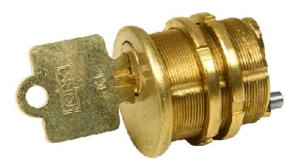
The Type CN22 (part# KC40---10) is a threaded cylinder interlock, commonly installed on circuit breaker interlocking kits. The cam on the back of the cylinder is made to interact with existing linkage on your equipment. The key is trapped or released according to the position of the cam. The CN22 can be linked to other CN22s with the proper bracketry.
